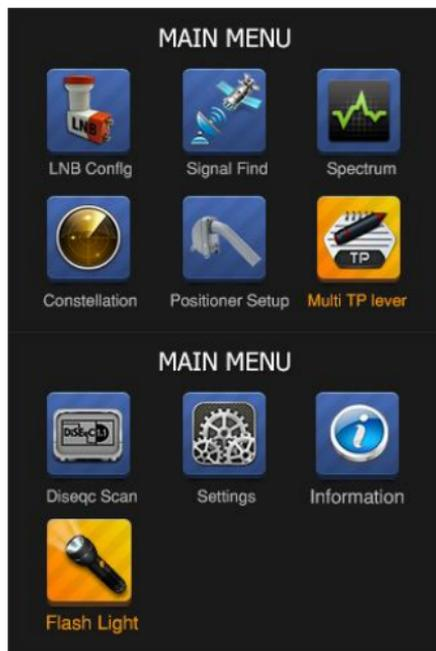
Navigate with the arrow keys (right, left, up and down) to select the desired function and confirm the selection with the OK button.
