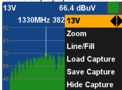
3. Save and load the capture for comparing the trail of Spectrum.
