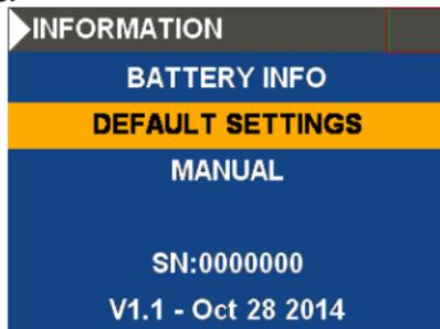
To protect against accidental resetting of the device, you receive a confirmation prompt here whether the device should really be set to factory defaults.
