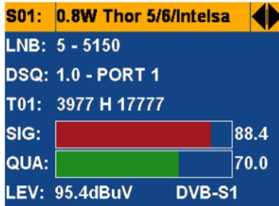
1. Press OK to display signal information, such as level, Carrier/Noise ratio and the Bit/Error rate.
