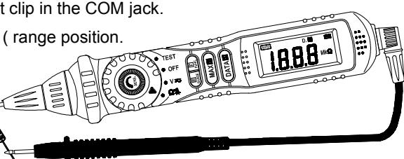
4.9.4 Connect the probe tip of the meter to one side of the tested circuit and probe tip of the test lead (or test clip) to the other side.
