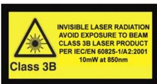
Additional laser safety information can be found on the Optek website. See application bulletin #221. Classification is not marked on the device due to space limitations. See package outline for centerline of optical radiance. Operating devices beyond maximum rating may result in hazardous radiation exposure.
