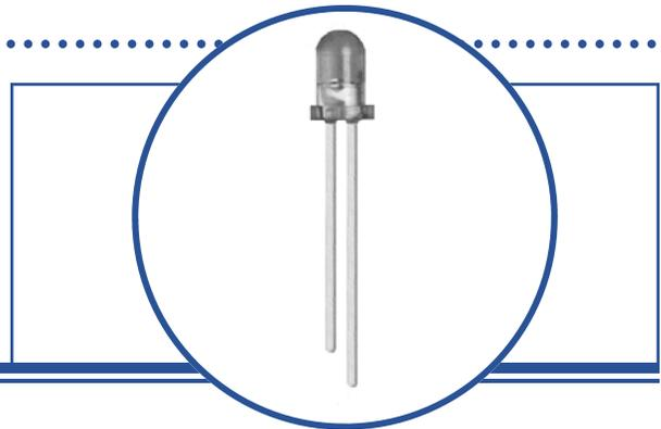
The OPV332 is a Vertical Cavity Surface Emitting Laser (VCSEL) packaged in a dome lens T-1 package. VCSELs offer many advantages in sensing applications when compared to infrared LEDs. These devices require substantially lower drive currents to obtain the same amount of output power as LEDs. This feature allows VCSELs to be used in low power consumption applications such as battery operated equipment.
