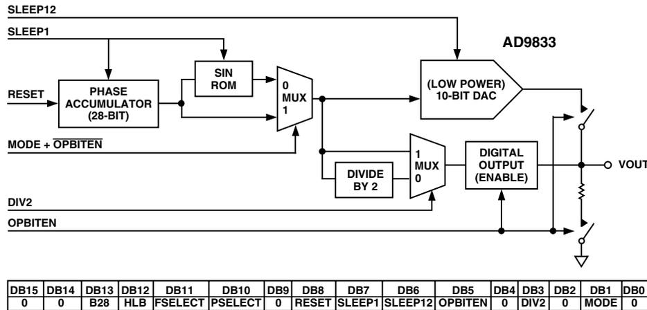
*Figure 5. Function of Control Bits*
