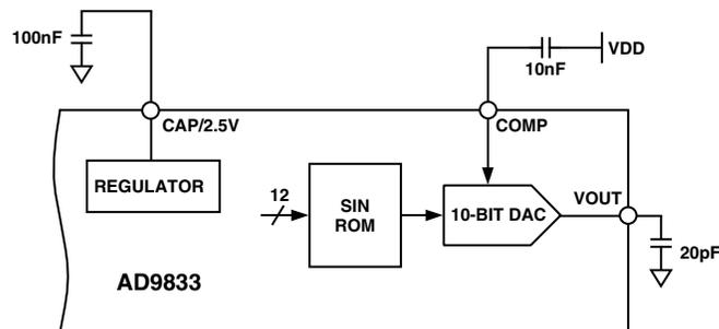
Figure 1. Test Circuit Used to Test Specifications
