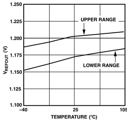
TPC 8.  $V_{REFOUT}$  vs. Temperature
