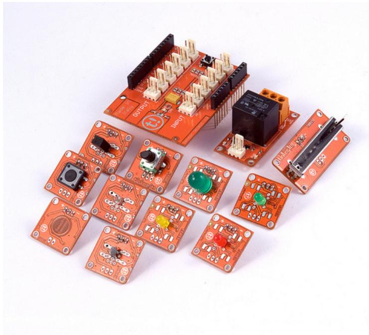
The **Base Kit** is a pack of different TinkerKit Modules, aimed to start designing interactive environments / prototype interfaces without using the breadboard or the soldering iron.
