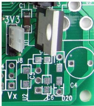
**Fig. 7: Image showing header J7 with translucent jumper in place. J7 is located just above J8 (J7 legend is obscured in this image)**
