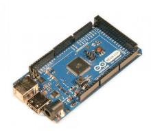
The Arduino ADK R3 is a microcontroller board based on the ATmega2560 (<u>datasheet</u>). It has a USB host interface to connect with Android based phones.
