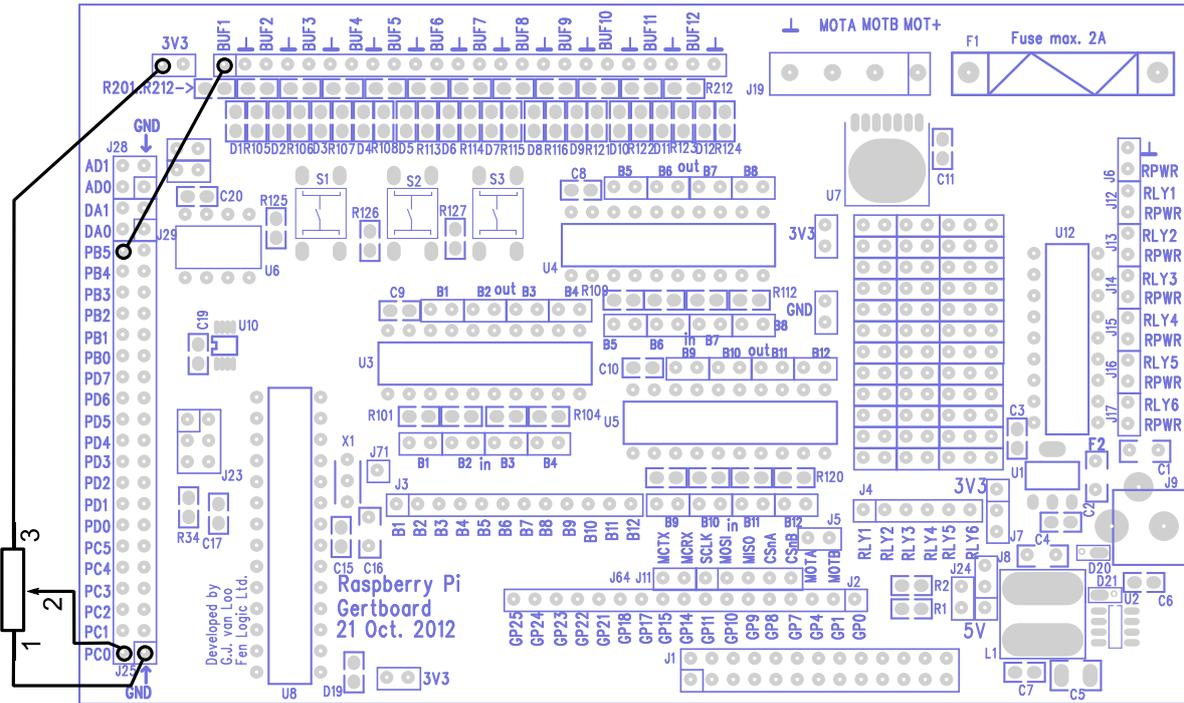
Figure 32: Wiring diagram for the AnalogInput sketch.
