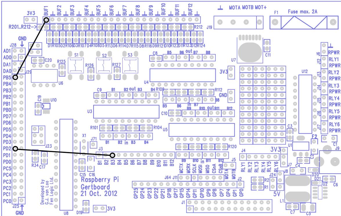
Figure 31: Wiring diagram for the sketch Button.
