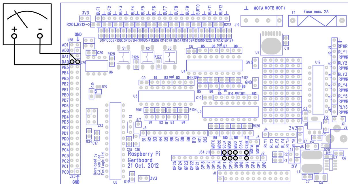
Figure 22: The wiring diagram for the dtoa test.
