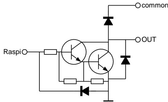
**Figure 15: Circuit diagram of each open collector driver.**
