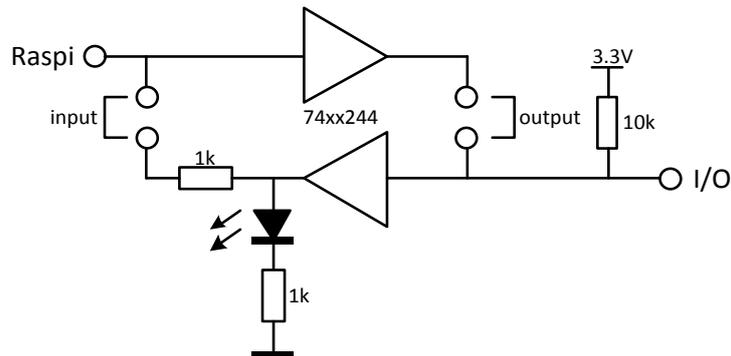
**Figure 8: The circuit diagram for I/O ports 4-12.**
