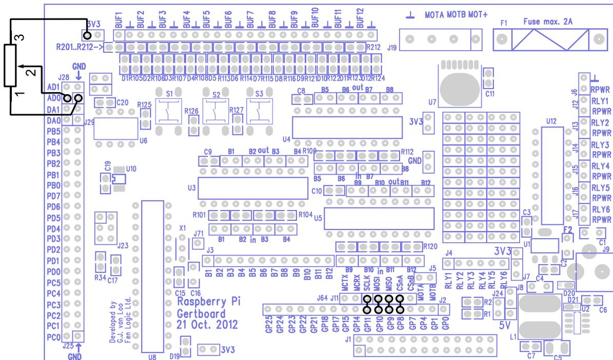
**Figure 23: Wiring diagram for the test program `atod`.**
