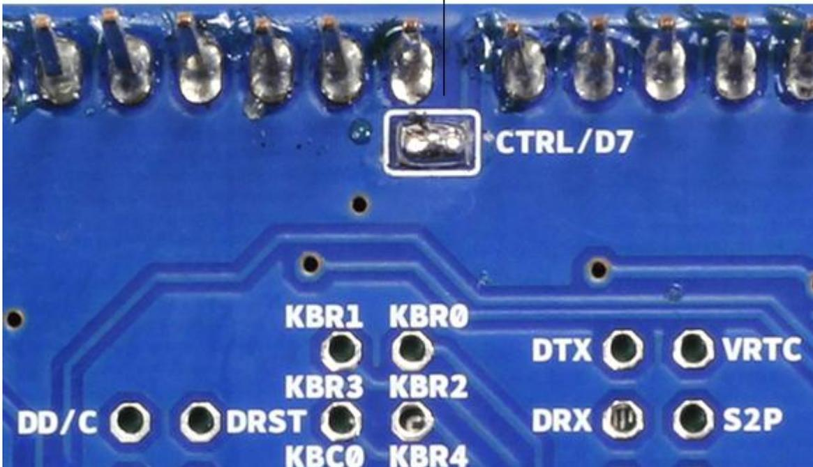
Several of the modem pins are exposed on the underside of the board. These provide access to the modem for features like speaker output and microphone input. See the datasheet for complete information.
