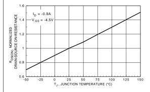
Figure 3. On-Resistance Variation with Temperature.
