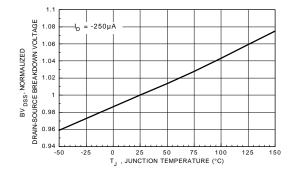
Figure 7. Breakdown Voltage Variation with Temperature.
