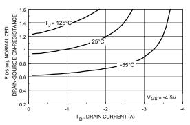
Figure 4. On-Resistance Variation with Drain Current and Temperature.
