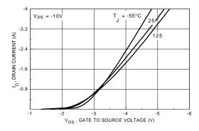
Figure 5. Transfer Characteristics.
