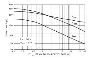
Figure 9. Capacitance Characteristics.
