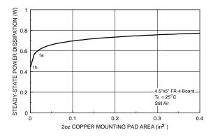
Figue 15. SuperSOT<sup>™</sup>-3 Maximum Steady-State Power Dissipation versus Copper Mounting Pad Area.
