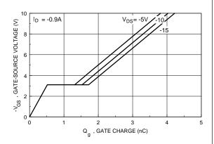
Figure 10. Gate Charge Characteristics.
