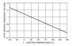
Figure 6. Gate Threshold Variation with Temperature.
