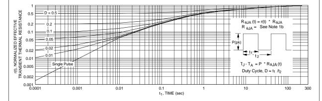
Figure 17. Transient Thermal Response Curve.
