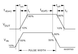
Figure 12. Switching Waveforms.
