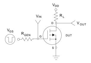
Figure 11. Switching Test Circuit.
