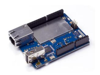
text based formats like XML that require quite a lot or ram to parse. On the Arduino YÚN we have created the Bridge library which delegates all network connections and processing of HTTP transactions to the Linux machine.
