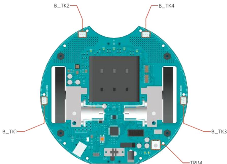
**Serial Communication:** The boards communicate with each other using the processors' serial port. A 10-pin connector connects both boards carries the serial communication, as well as power and additional information like the battery's current charge.
