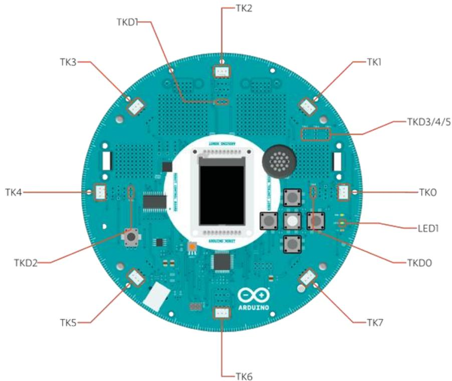
**Motor Board TK1 to TK4:** these pins are named in software as **B\_TK1** to **B\_TK4**, they can be digital or analog input pins, and support Robot.digitalRead(), Robot.digitalWrite() and Robot.analogRead().
