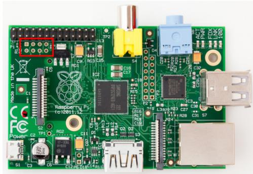
**Diagram 2: Raspberry Pi with P5 connector outlined in red**
