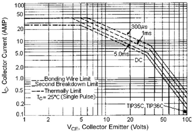
There are two limitations on the power handling ability of a transistor: average junction temperature and second breakdown safe operating area curves indicate  $I_C$ - $V_{CE}$  limits of the transistor that must be observed for reliable operation i.e., the transistor must not be subjected to greater dissipation than the curves indicate.
