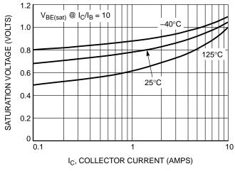
Figure 7. D44H11 ON-Voltage
