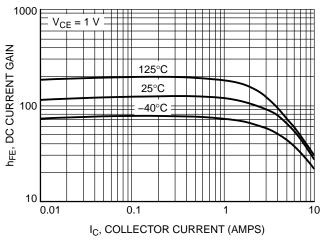
Figure 2. D45H11 DC Current Gain
