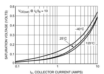
Figure 6. D45H11 ON-Voltage
