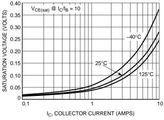
Figure 5. D44H11 ON-Voltage
