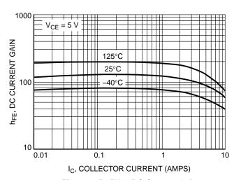
Figure 4. D45H11 DC Current Gain
