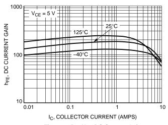
Figure 3. D44H11 DC Current Gain
