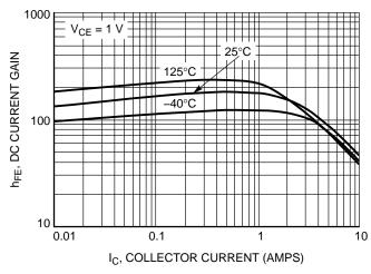
Figure 1. D44H11 DC Current Gain
