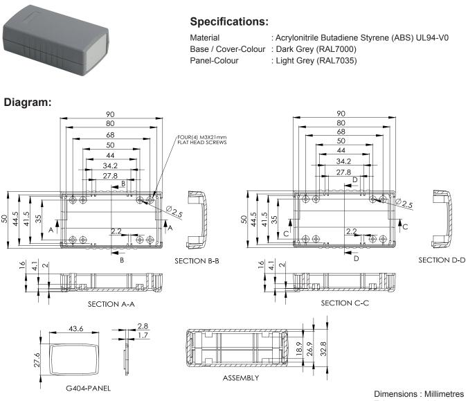
Dimensions : Millimetres Tolerances :± 0.3mm
