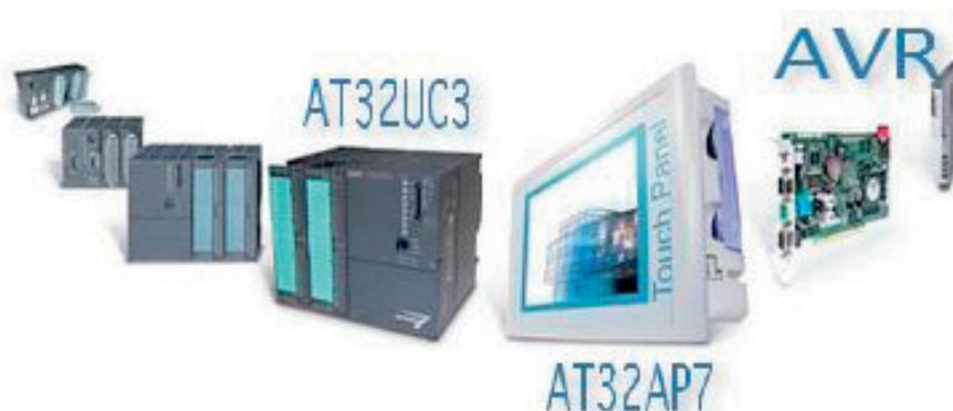
The core of the AT32AP7 family is attached to a Vector-Multiplication-Unit (Pixel Coprocessor) which may be used to scale or rotate images as well as for color conversion algorithm. The embedded LCD controller supports STN and TFT display up to 2048x2048 pixel resolution at 8 pixels per color. Several other media interfaces like Audio Codec's, Multimedia Card and high-speed USB device interfaces opens a wide range of applications needed in consumer, automotive and industrial areas.
