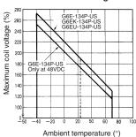
The maximum coil voltage refers to the maximum value in a varying range of operating power voltage, not a continuous voltage.
