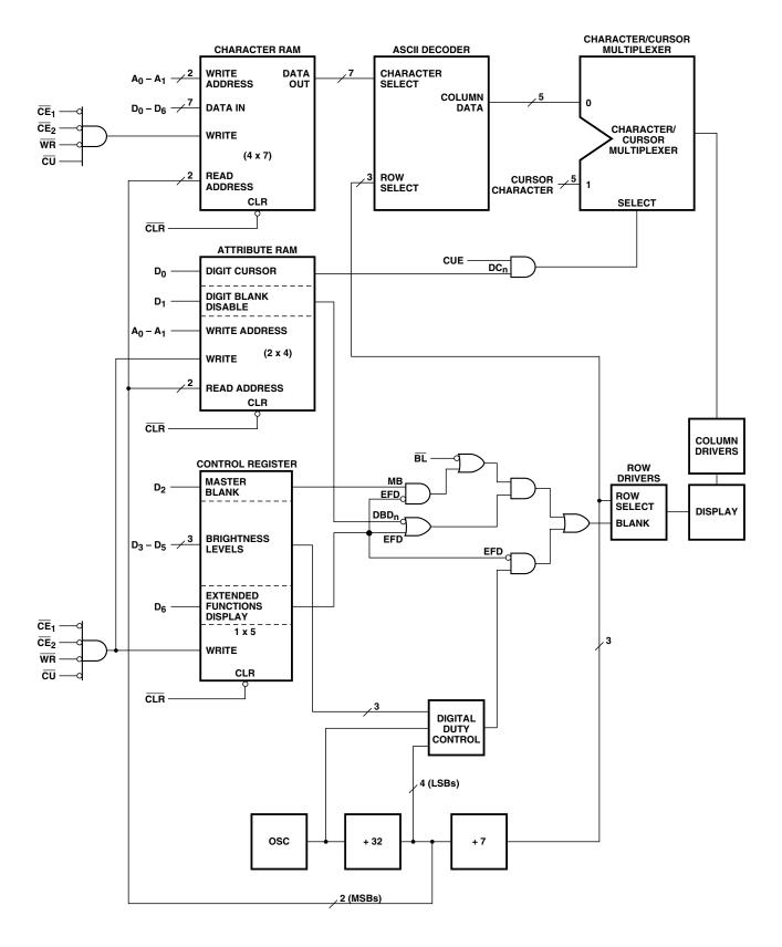
Figure 1. Internal block diagram.
