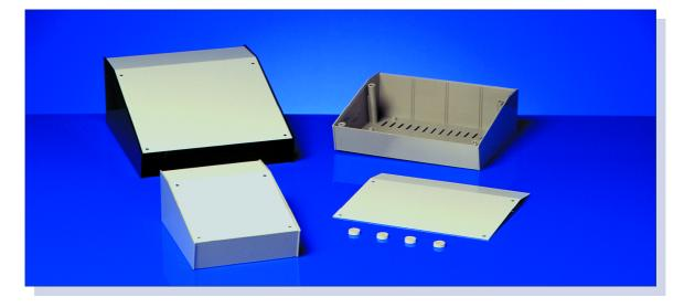
The 6000 range of small desk consoles are of a two piece construction. They incorporate 1mm thick, grey aluminium front panels which sit recessed into the top of the ABS bases and are held by four fixing screws running into integral brass inserts.
