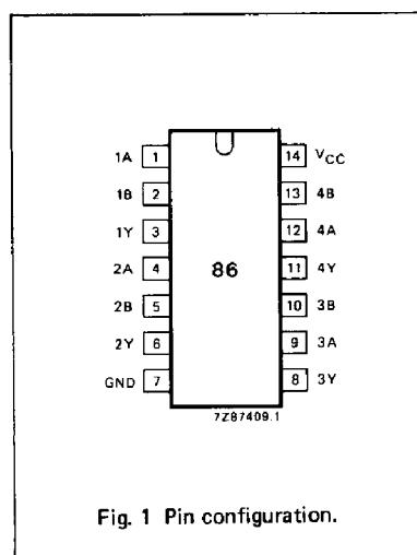
Fig. 1 Pin configuration.
