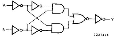
Fig. 5 Logic diagram (one gate).
