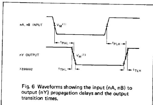
Fig. 6 Waveforms showing the input (nA, nB) to output (nY) propagation delays and the output transition times.
