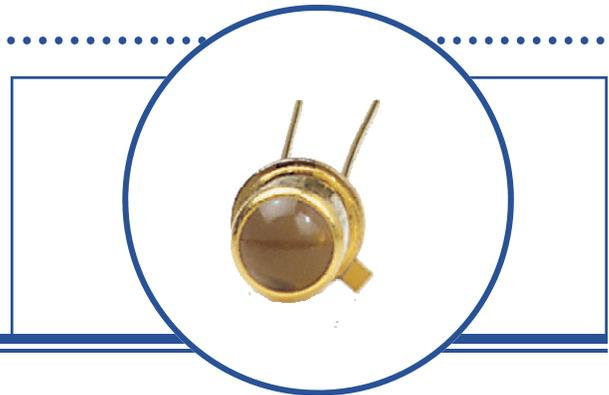
The OPV302 is a Vertical Cavity Surface Emitting Laser (VCSEL) packaged in a dome lens TO-46 package. VCSELs offer many advantages in sensing applications when compared to infrared LEDs. These devices require substantially lower drive currents to obtain the same amount of output power as LEDs. This feature allows VCSELs to be used in low power consumption applications such as battery operated equipment.
