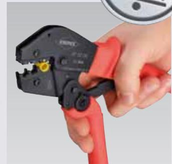
**First step:** move the handle with two fingers only until both jaws touch the connector to be crimped
