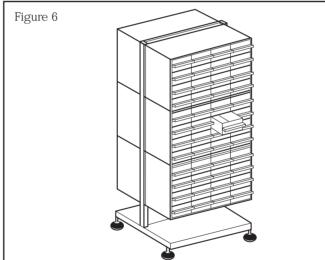
Note: Whilst under normal circumstances the assembled framework will be stable, care should be taken to ensure that the weight of the stored items is evenly distributed with heavier items located at the bottom.
