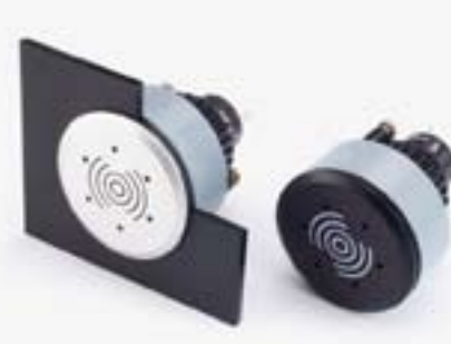
Buzzer, flush mount, 30.5 mm mounting, IP40, 24 VDC, 95dB ±8 at a distance of 0.1m
