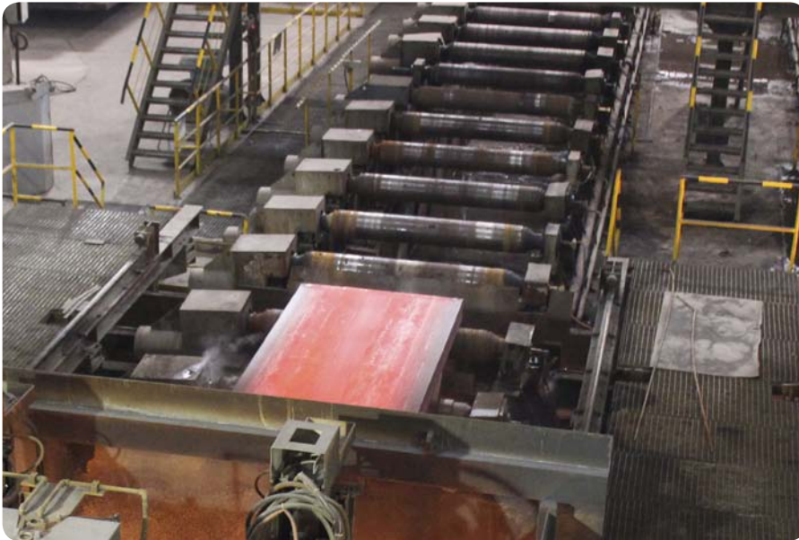
Roll-out table transporting slabs from a continuous casting machine.
