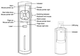
A) When the switch is put on "KEYBOARD", it functions as a wireless keyboard as below:
