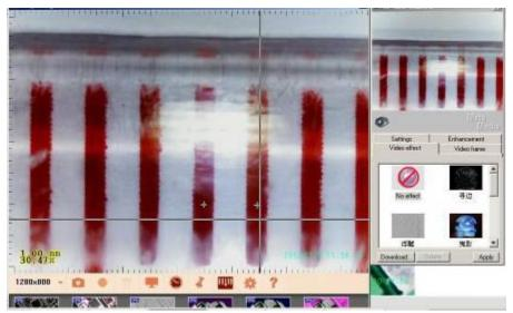
Click on the ruler by two points. These points are marked as "+" and the distance of these points on the ruler should be 1 mm or 10 mm as you select the unit on the pop-up menu.
