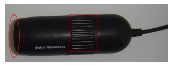
In the figure, a red box shows the focus ring of the microscope camera. The lens side of the microscope camera is shown in a red oval line. This end should be closer to the object for getting a large magnification view.
