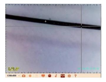
Now, we can measure the distance between two points on a hair of 0.84mm. (Note that if you change the position of microscope camera, you will need to do the calibration again, because the magnification factor is different.)
