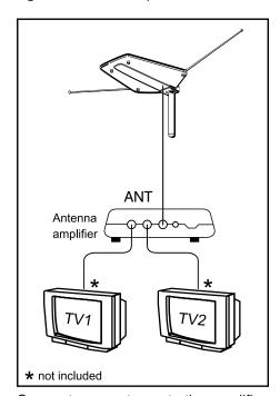
Connect your antenna to the amplifier, and the amplifier to one or two TVs.
