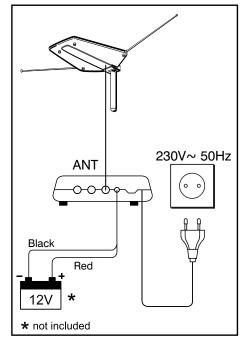
Plug the amplifier into a wall outlet or use the red and black cable for the power supply of the amplifier by a car battery\*.
