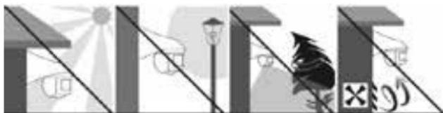
6. Attach the cover cap to a wall or ceiling in a height of 1.8 to 2.5 m with the installation material. At this, attend to the cable location and its lateral alignment. The detection area is 180° in a distance of max. 12 m.
