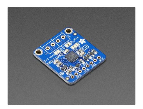
However, to get that precision and accuracy out of your PT100x RTD you must use an amplifier that is designed to read the low resistance. Better yet, have an amplifier that can automatically adjust and compensate for the resistance of the connecting wires. If you're looking for a great RTD sensor, today is your lucky day because we have a lovely Adafruit RTD Sensor Amplifier with the MAX31865 sensor.
