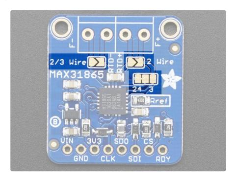
By default the sensor is wired up for 4-wire RTD usage but can be set up for 2 or 3 wire very easily.
