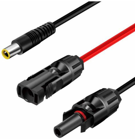
The solar adapter cable (DC7909 to MC4) is a special cable used to connect solar panels with an MC4 connector to a power station with a DC7909 connector. The MC4 connectors are widely used in the solar industry and provide a reliable and safe connection for the transmission of direct current. It enables clean solar energy to be transmitted and utilised.
