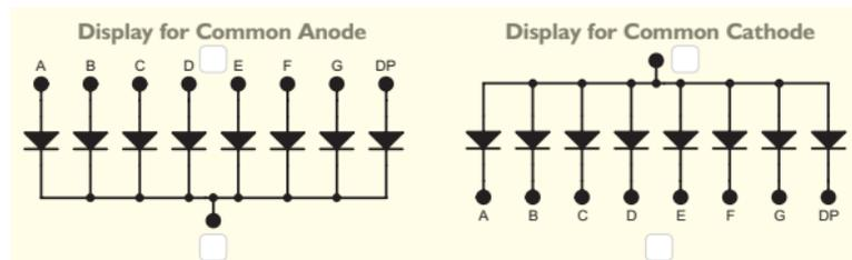
The practice N°1 allows to shows different power supplies and the segments control according to the display type; common cathode or anode. The goal of this practice is to identify the power supply polarisation of the display as well as the control input one for each segment regarding the common cathode or anode configuration.
