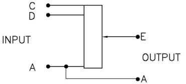
Connection 230V on A – C delivers max. 230V output A – E.
