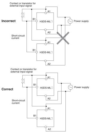
The H3DS Series is provided with a transformerless power supply system.
