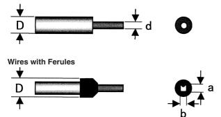
Note: 1. If the overall diameter of the wire is less than 1.8 mm, do not insert the wire past the conductor. Refer to the following diagrams.
