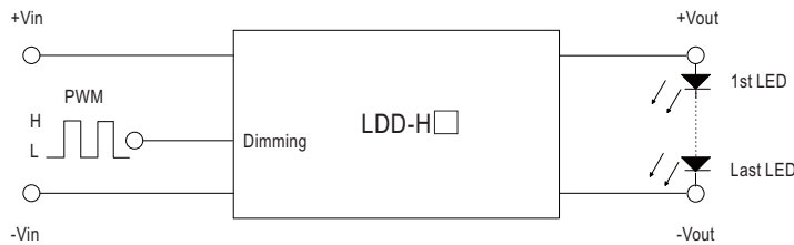
Fig-1 12VDC input, 1~3 LEDs(Vf=3V)
