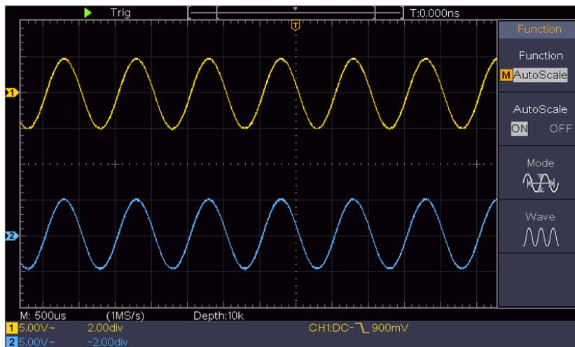
Figure 4-12: Autoscale Horizontal-Vertical multi-period waveforms
