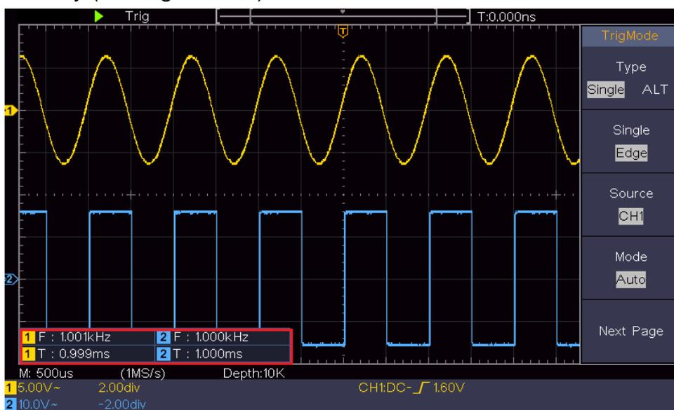
Figure 4-13 Automatic measurement
