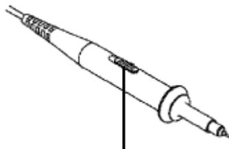
Figure 3-8 Attenuation Switch
