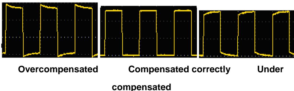
Overcompensated      Compensated correctly      Under compensated
