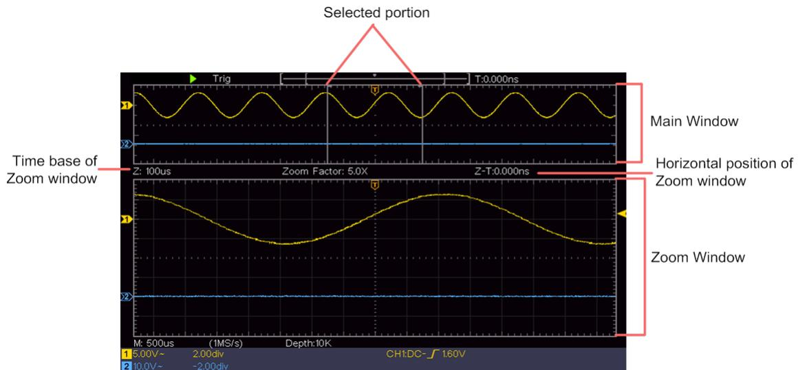
In normal mode, the **Horizontal Position** and **Horizontal Scale** knobs are used to adjust the horizontal position and time base of the Main window. In wave zoom mode, the **Horizontal Position** and **Horizontal Scale** knobs are used to adjust the horizontal position and time base of the Zoom window.
