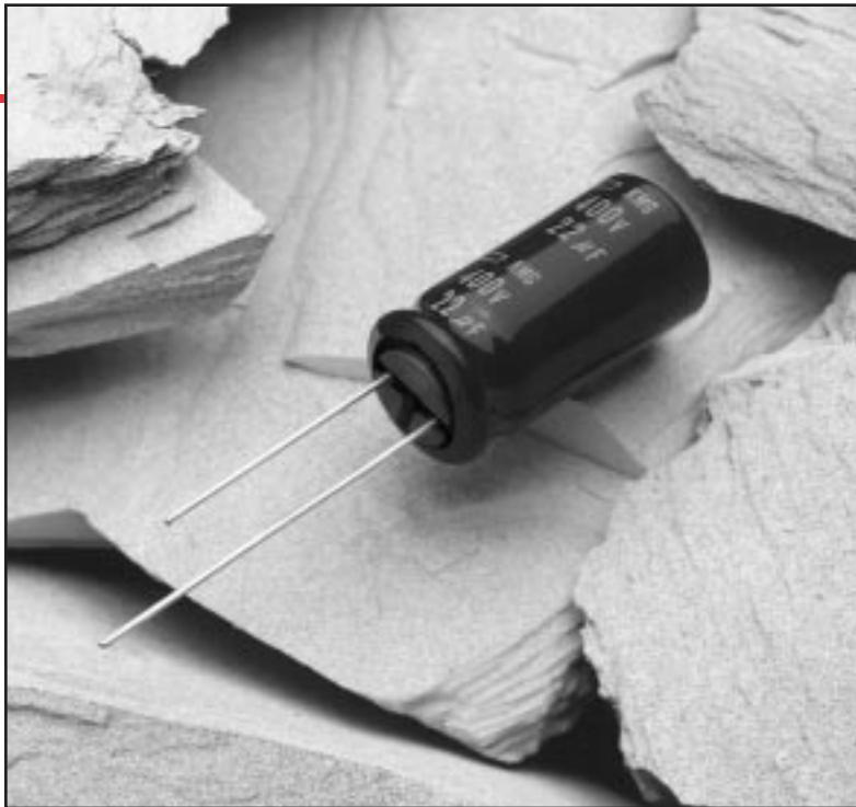
The KMG series capacitors are designed for general purpose use with an operating temperature range for most of these capacitors from  $-55^{\circ}\text{C}$  to  $+105^{\circ}\text{C}$ . The KMG series is a miniaturized version of the KME series with a load life of 1,000 hours at  $105^{\circ}\text{C}$  with the rated ripple current applied.
