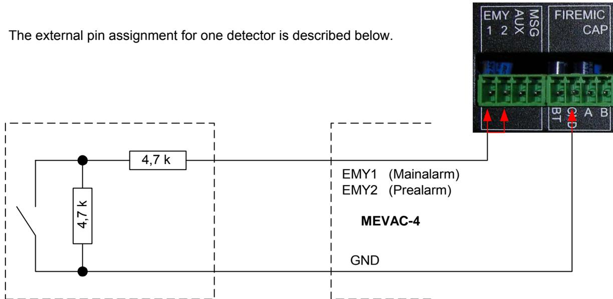
In case of several detectors to be connected to one alarm connection, they are connected together as follows. A series connection is compulsory.
