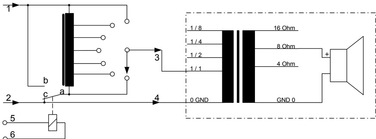
When the control is set to its maximum position at the installation run and is then turned to 50 % during operation, it will be identified as a deviation of more than 20 % and a corresponding error message will be displayed. In case the attenuator is in operation during the installation run, the connected speaker circuit may be identified as uninstalled.
