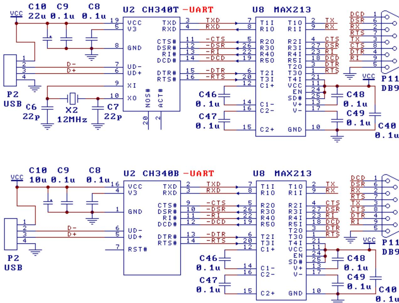
The image above use CH340T/CH340B (or CH340C ) to realize USB to RS232 converter. CH340 provides common UART and MODEM signals, converts TTL to RS232 through level conversion chip U8. Port P11 is DB9 connector, the pins and their functions are the same as common PC DB9 connector, the chips similar with U8 have MAX213/ADM213/SP213/MAX211 etc.
