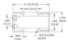
Holds any size, any shape, standard 9 Volt battery. Eliminates need to specify an exact battery brand, size or shape. Ideal for power source or memory back-up use in PLC, telecommunications, data processing, security systems, clocks, radios, toys and appliances.
