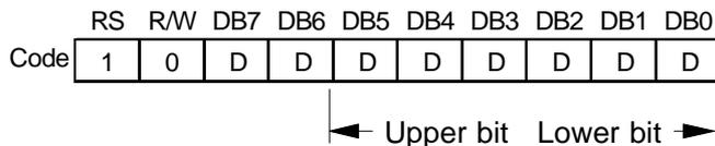
Binary eight-bit data DDDDDDDD is written into CG RAM or DD RAM. CG RAM Address Set or DD RAM Address Set before this instruction selects either RAM. After the write operation, the address is incremented or decremented automatically according to Entry Mode Set. Entry Mode Set also determines whether display shifts or not after the write operation.
