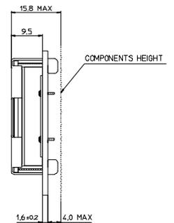
Note : Only dimension changes between Reflective/EL and LED backlight is thickness.
