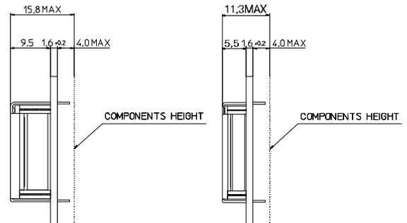
Note : Only dimension changes between Reflective/EL and LED backlight is the thickness
