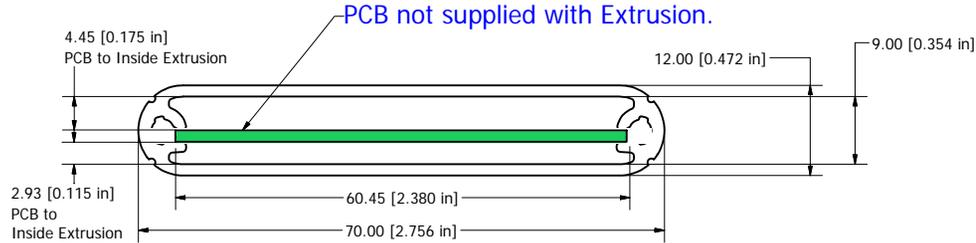
Extrusion designed for 60mm wide x 100mm long PCBs.
