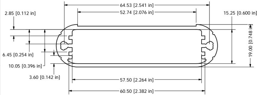
Extrusion designed for 60mm wide x 100mm long PCBs.
