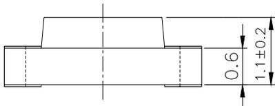
For reflow soldering (propose)
