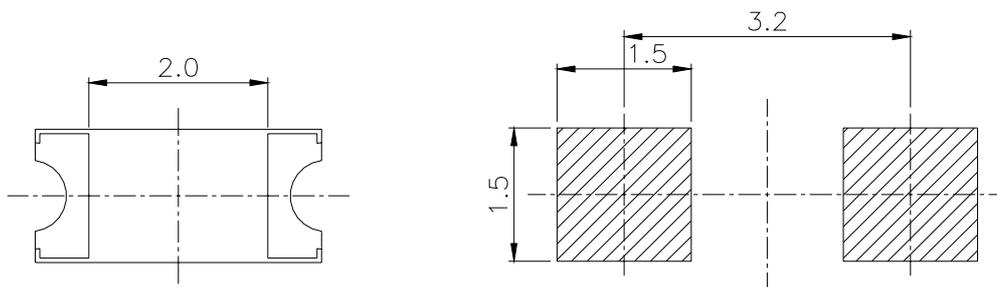
**Note:** Tolerances Unless Dimension  $\pm 0.1\text{mm}$  , Unit = mm
