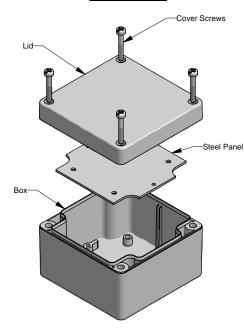
NOTE Purchased assembly includes box, lid and 4 cover screws. Cover screws should be torqued to 2.5 lbf-in (30 cN-m) Polycarbonate version is \$\infty\$508 approved Enclosure Type 4X, 4, 12 File# E65324
