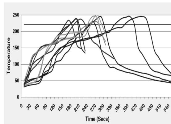
**Illustration:** Soldering profile recommended by the manufacturer Alpha-Metals for paste OMNIX OM 338. For KFS 140, the peak temperature must be below 240°C at approx. 1-minute peak hold time.
