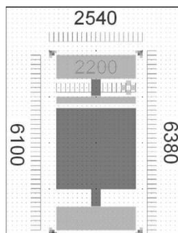
**Illustration:** Chip geometry of the SMD-Humidity sensors in µm
