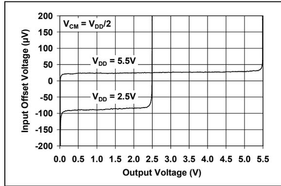
**FIGURE 2-10:** Input Offset Voltage vs. Output Voltage.
