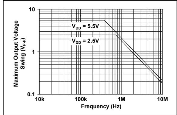
**FIGURE 2-28:** Maximum Output Voltage Swing vs. Frequency.
