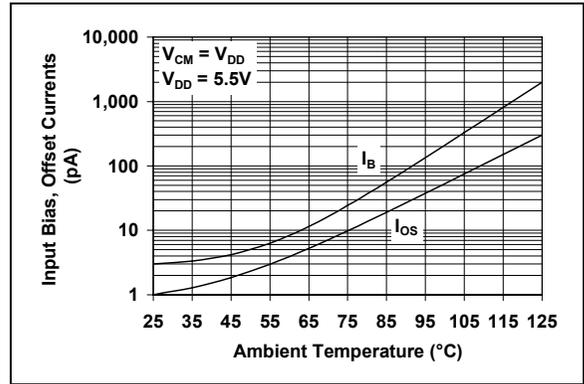
**FIGURE 2-16:** Input Bias, Offset Currents vs. Temperature.
