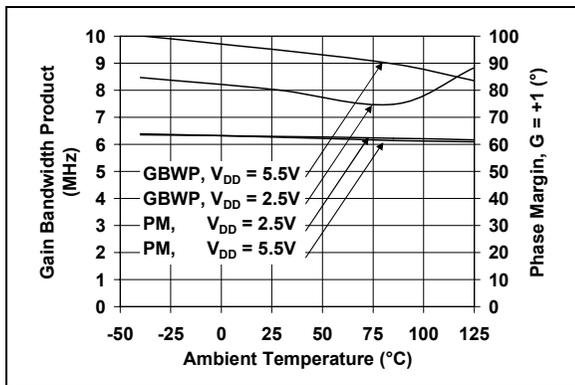
**FIGURE 2-21:** Gain Bandwidth Product, Phase Margin vs. Temperature.
