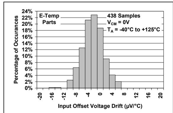
**FIGURE 2-5:** Input Offset Voltage Drift, (Extended Temperature Parts).
