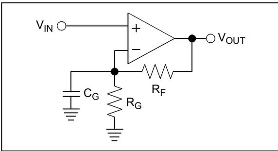
**FIGURE 4-4:** Non-inverting gain circuit with parasitic capacitance.
