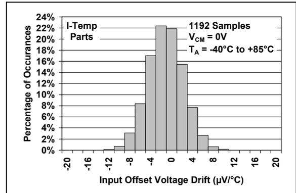
**FIGURE 2-4:** Input Offset Voltage Drift, (Industrial Temperature Parts).
