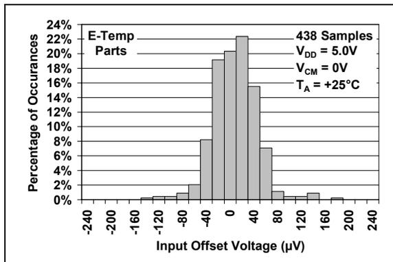
**FIGURE 2-2:** Input Offset Voltage, (Extended Temperature Parts).
