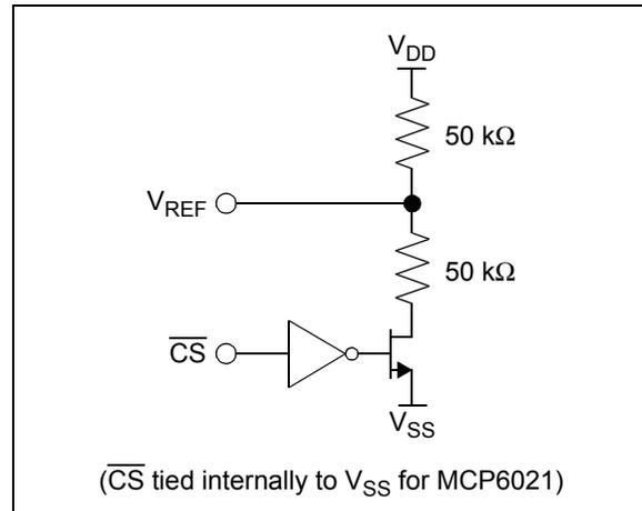
**FIGURE 4-6:** Simplified internal  $V_{REF}$  circuit (MCP6021 and MCP6023 only).
