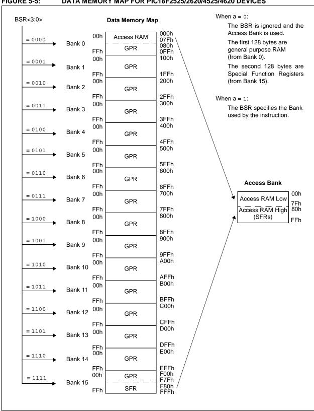
FIGURE 5-5: **DATA MEMORY MAP FOR PIC18F2525/2620/4525/4620 DEVICES**
