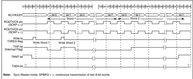
FIGURE 18-12: SYNCHRONOUS TRANSMISSION (THROUGH TXEN)
