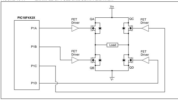
FIGURE 16-7: EXAMPLE OF FULL-BRIDGE APPLICATION
