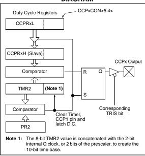
A PWM output (Figure 15-4) has a time base (period) and a time that the output stays high (duty cycle). The frequency of the PWM is the inverse of the period (1/period).
