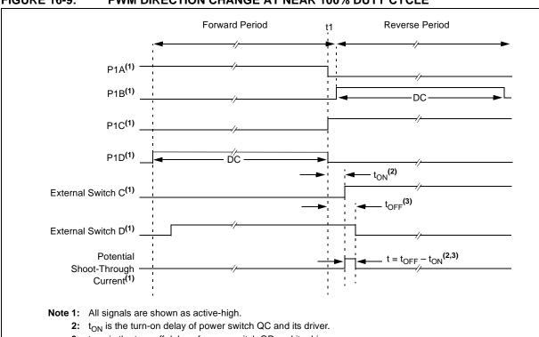
3: t<sub>OFF</sub> is the turn-off delay of power switch QD and its driver.
