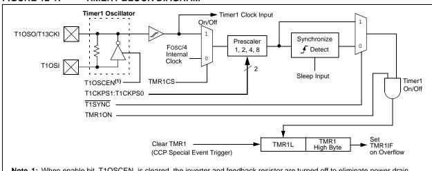
Note 1: When enable bit, T10SCEN, is cleared, the inverter and feedback resistor are turned off to eliminate power drain.
