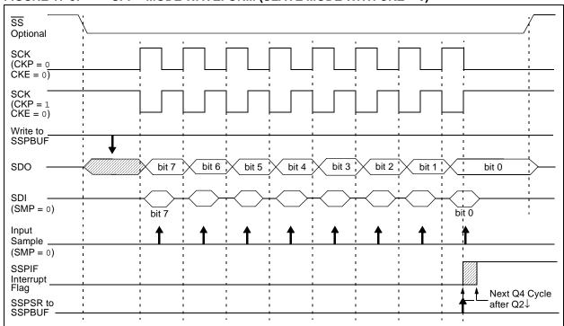
FIGURE 17-6: SPI™ MODE WAVEFORM (SLAVE MODE WITH CKE = 1)
