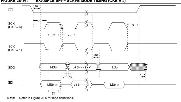
FIGURE 26-16: EXAMPLE SPI™ SLAVE MODE TIMING (CKE = 1)
