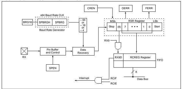
FIGURE 18-7: ASYNCHRONOUS RECEPTION
