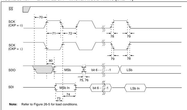
FIGURE 26-13: EXAMPLE SPI™ MASTER MODE TIMING (CKE = 0)
