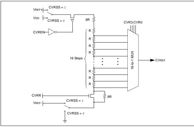
FIGURE 21-1: COMPARATOR VOLTAGE REFERENCE BLOCK DIAGRAM
