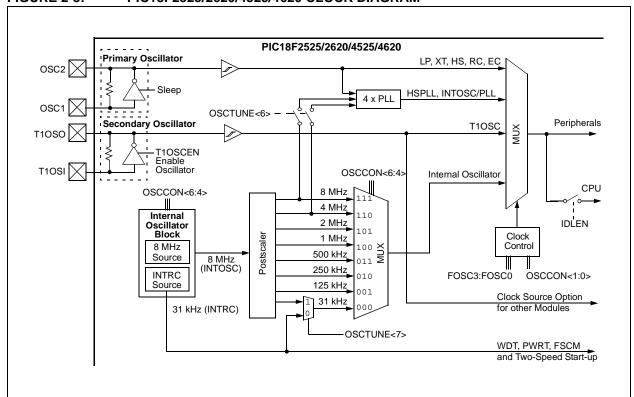
FIGURE 2-8: PIC18F2525/2620/4525/4620 CLOCK DIAGRAM
