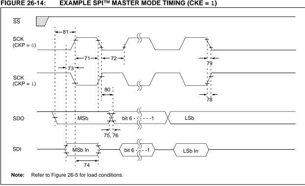
FIGURE 26-14: **EXAMPLE SPI™ MASTER MODE TIMING (CKE = 1)**
