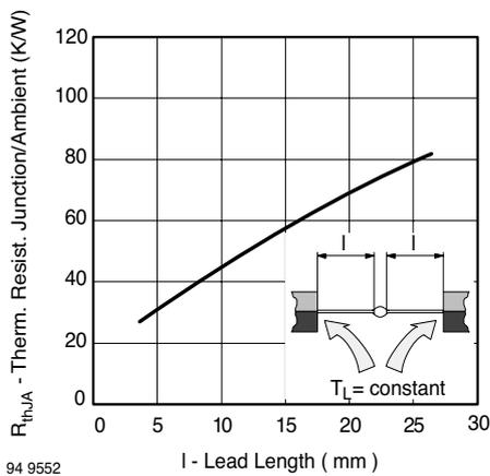
Figure 1. Max. Thermal Resistance vs. Lead Length
