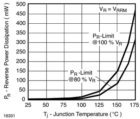
Figure 5. Max. Reverse Power Dissipation vs. Junction Temperature
